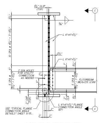
INTERMEDIATE STIFFENER WITH FLANGE CONNECTION ANGLE
